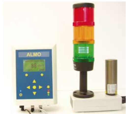
ALMO 1 with GM-probe and 3-level LED-lamp
