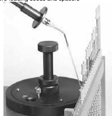
The SeedVac™ hand piece with the clear tube tips used for pre-loading seeds and spacers
