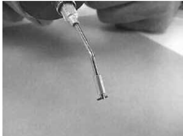
Picking up a single seed. Note the tip is centered on the seed.
