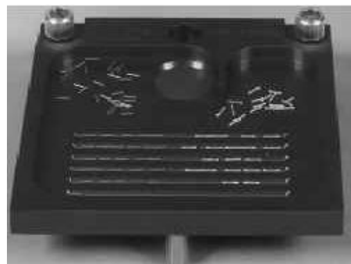
The Seed Alignment Tray with the seeds and spacers ready for loading.
