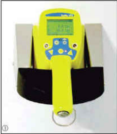
Stationary operation of CoMo-system in active wall station
