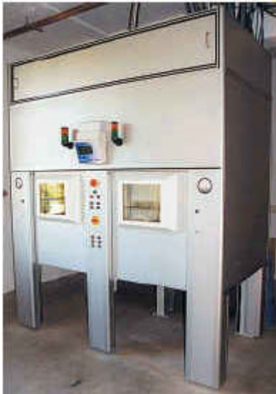
Example of a dose rate monitoring system with alarm units
