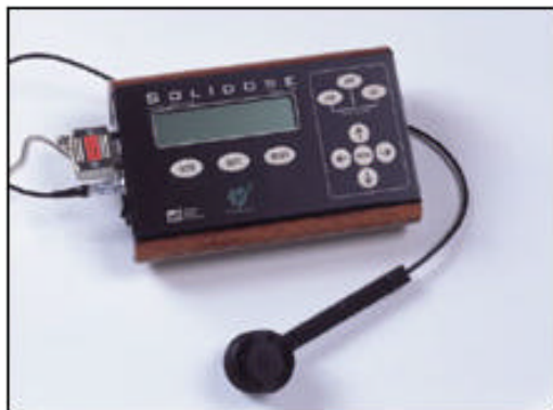
Solidose 400 with Magna ionization chamber
