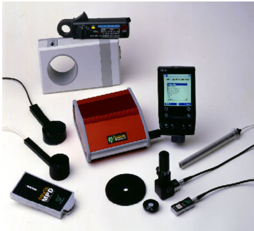
From ion chambers to mAs probes, the BARRACUDA supports them all. Also, owners of existing solid-state detectors and probes manufactured by RTI can use them with their new BARRACUDA.
